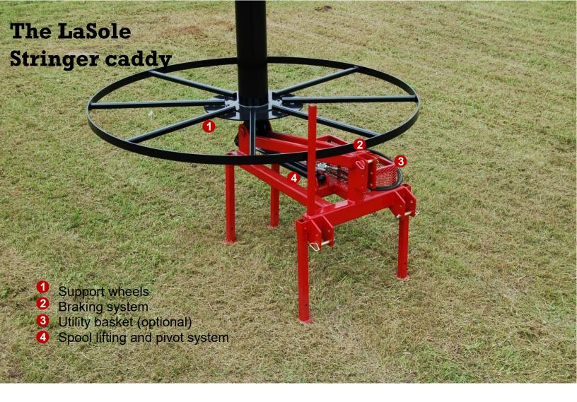
Carried on the tractor's 3-point hitch, the stringer caddy has great maneuverability. The support wheels located under the swivel base enforce the main axle. The ingenious braking system is incorporated into pivot/lifting tile spool system. The entire machine is built as we build our other products: simple, functional, robust and economical.
